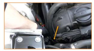
10. Separate the CCV hose from the intake manifold.
