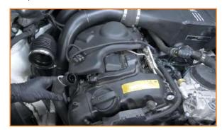
11. Disengage the electrical connector to release the heater block and CCV hose.
