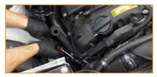
17. Install the smaller hose to the intake manifold.
