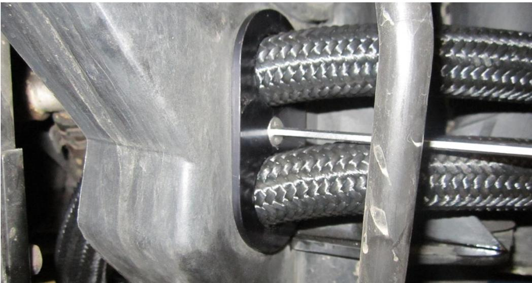
34. Place the oil hose clamp in position and tighten.
