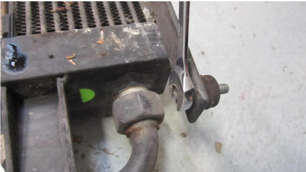
37. Place the lower Forge mounting bracket into position. Use the cotton reels just removed to attach at the back of the mounting plate. Please note the orientation of the plate as this is handed i.e. its offset to one side.
