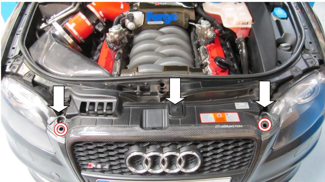
8. There are also some bumper height adjusters that should be loosened. This is not always necessary, but sometimes can help when you come to refit the bumper. These are circled in red.
