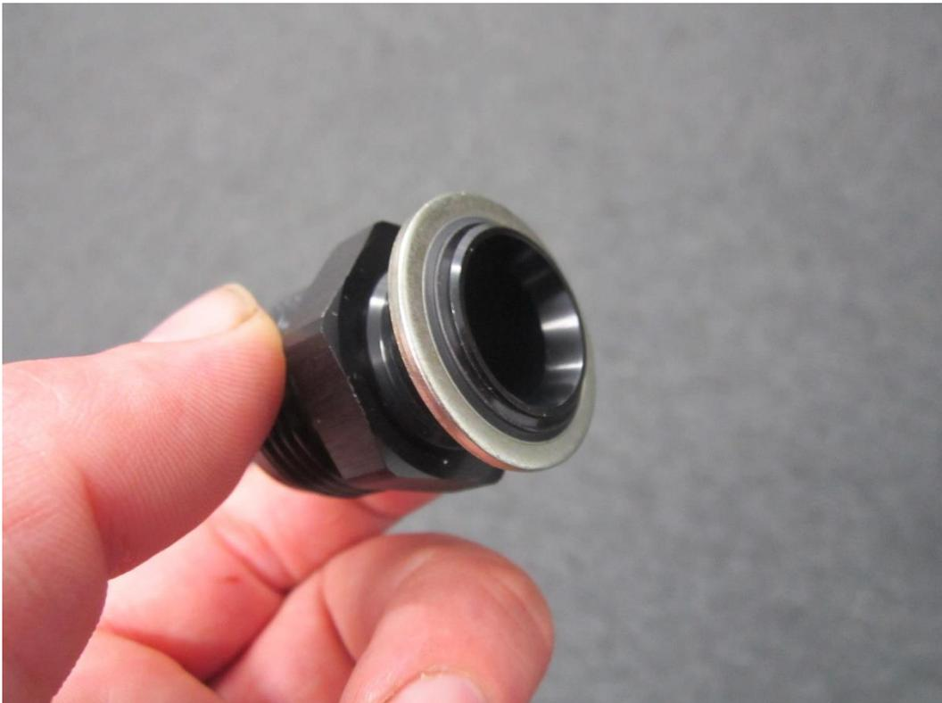
21. Now attach the M22 to dash 12 adaptor to the oil cooler, and using an adjustable spanner (or -12 spanner) tighten them down.
