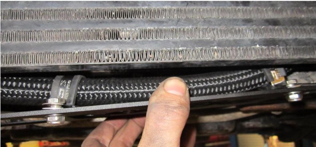
39. Using a 10mm spanner tighten all of the m6 nuts on all cotton reels and the two P clips.
