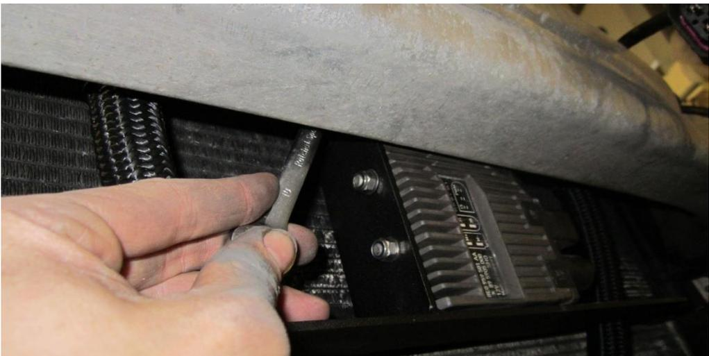
32. Connect the oil lines to the sandwich plate and tighten.
