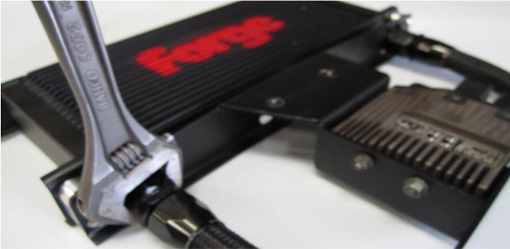
25. Tighten both of the oil lines using an adjustable spanner, or -12 spanner.
