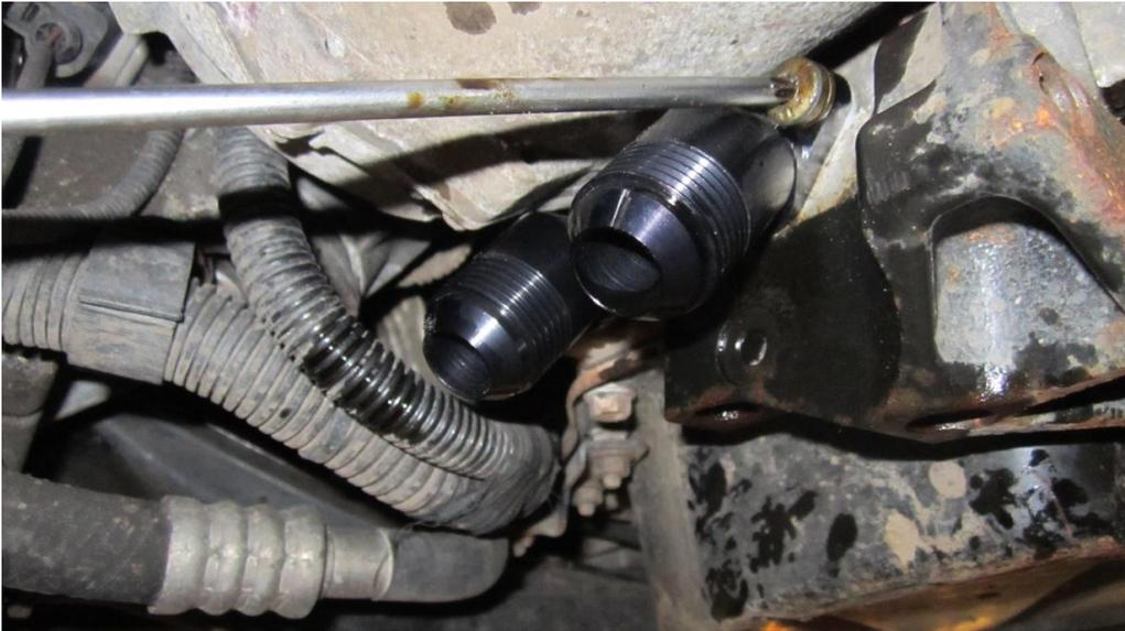
28. Slide the oil cooler assembly under and behind the crash bar into position.
