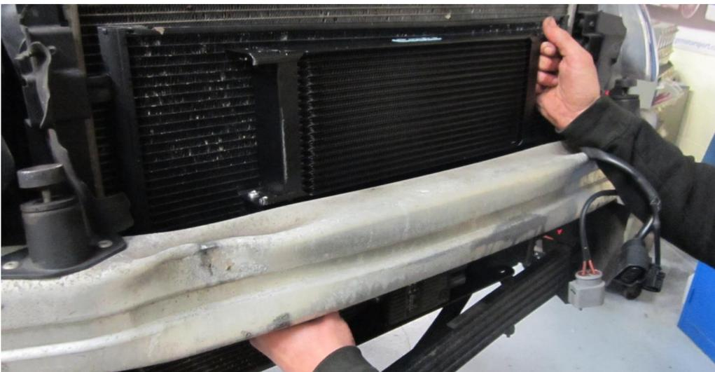
29. Using the two M6 hex heads removed in section 17 that held the fan controller bracket in position, attach the new assembly and tighten using a 10mm spanner.
