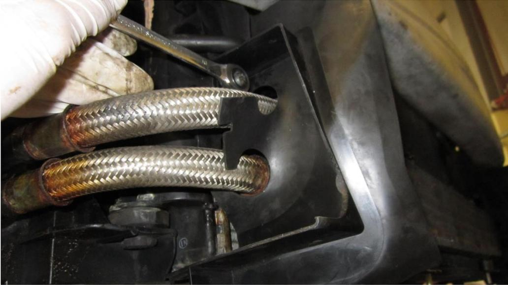
15. Now you will be able to slide out the cooler from between the radiator and the power steering cooler.
