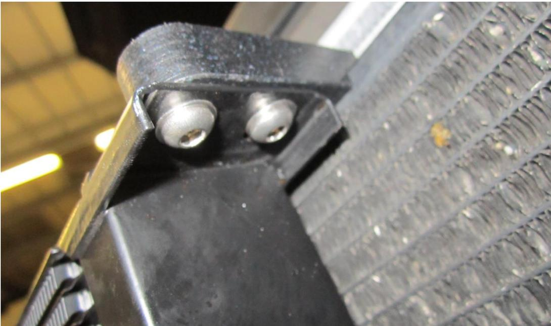
42. The new oil cooler kit is now fully assembled - make sure all fittings are tight. Add ONE litre of oil.
