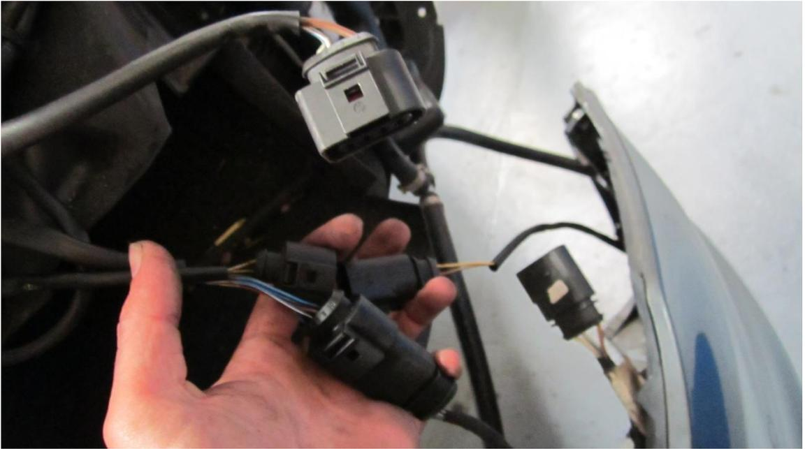
11. You also need to disconnect the washer jets, by pulling up the retainer and pulling out the hose. Have a jug ready to collect any screen wash you wish to keep.
