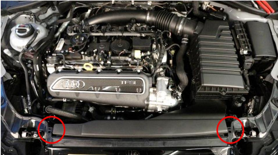
1. Remove the engine cover. Remove the 2 screws holding the inlet duct in place. Then push the duct into the airbox to release the mounting points and remove duct from engine bay.
