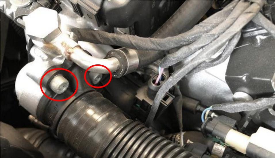
5. If you have a 2019+ vehicle with the above breather type please follow the next steps. If you have the breather system from step 3a please go to step 9. Remove the breather hose from the throttle body by removing these 2 screws.
