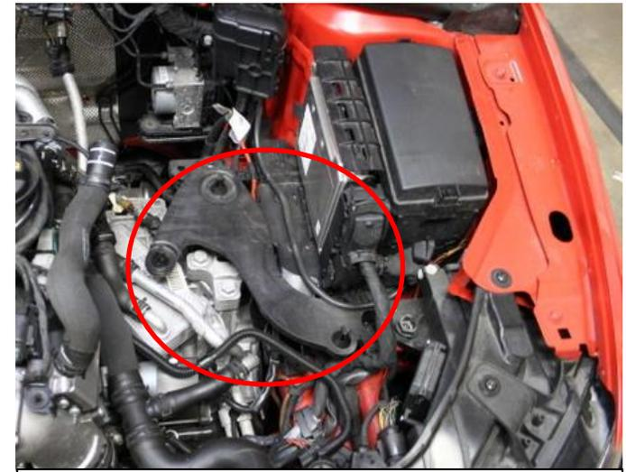
4. Remove entire airbox by pulling upwards. It is held in place with rubber push mounts. Also remove the Airbox mounting tray by unscrewing the 2 bolts.
