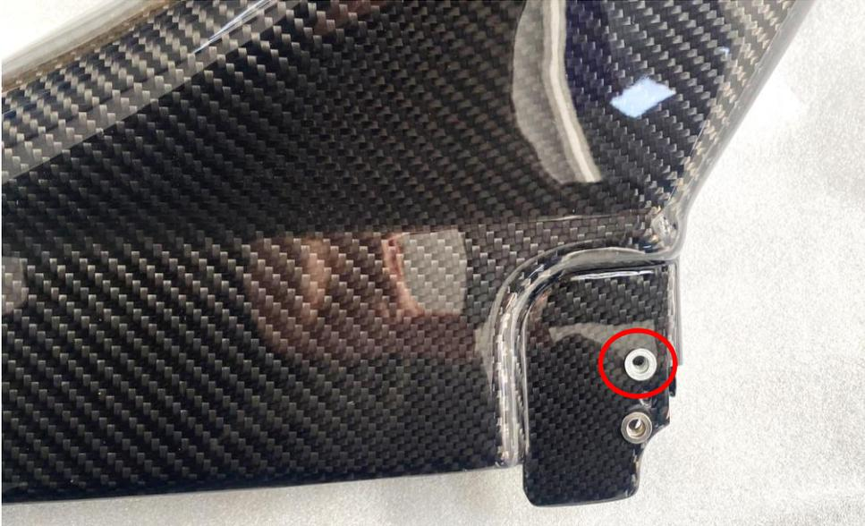
49. Before securing identify the correct holes to use on the duct. The upper threaded inserts as circled are to be used for the 8Y RS3.
