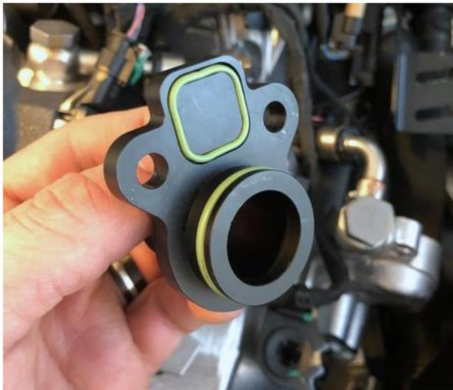
7. Install the seals into the new machined adapter fitting provided.
