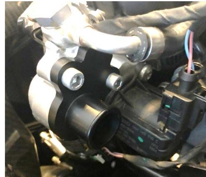
8. Install the adapter onto the throttle body with the original screws. Tighten to 9Nm.
