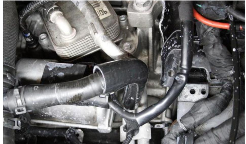
22. Push Hose 1 onto the tube which we rotated the clip on as shown.
