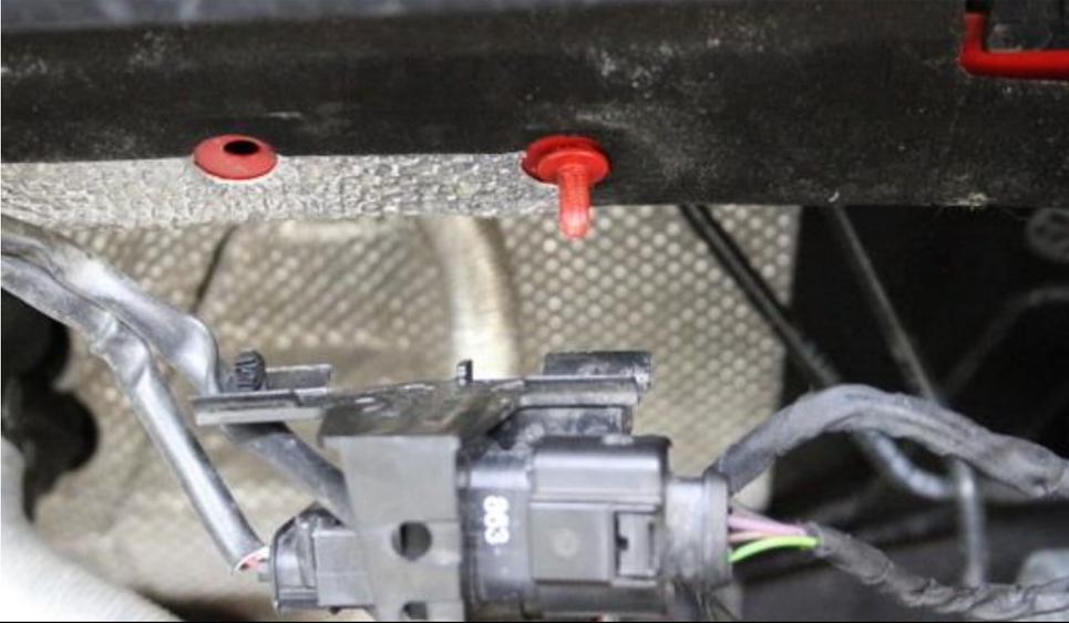
13. Remove the harness bracket from the chassis by using a small flat head screwdriver and carefully lever it off – one side is pushed onto a threaded stud and the other side has a plastic clip pushed into a hole on the chassis.
