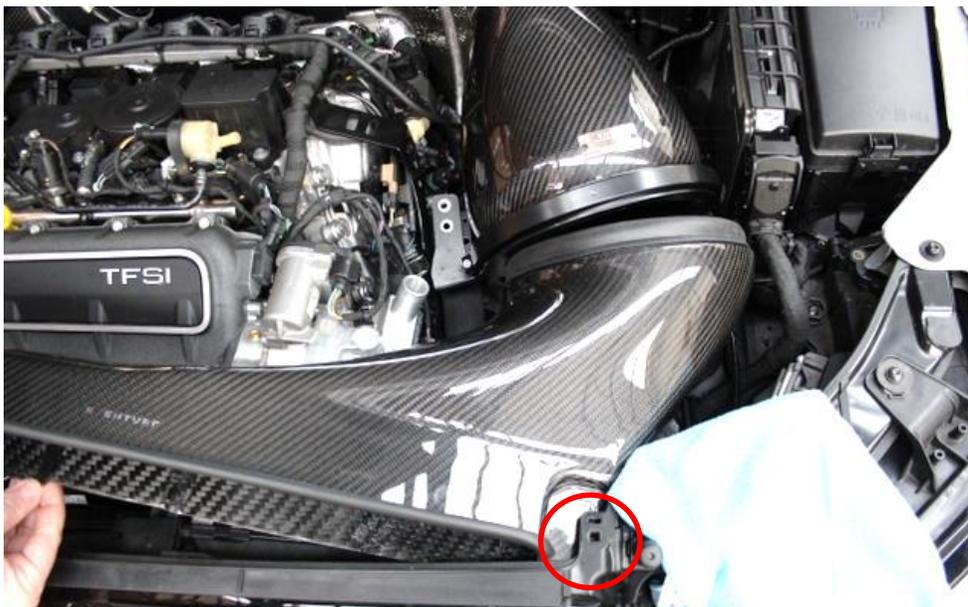
47. Now rotate the duct so the rear corner goes into the mounting location circled.
