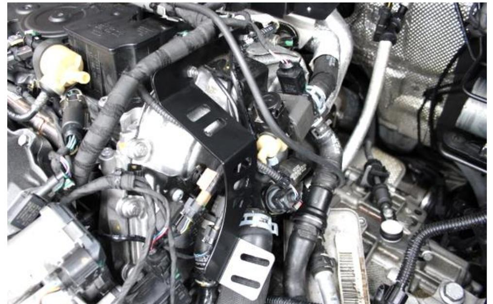
36. Place the new bracket into position as shown on top of the existing bracket. Use the lock nuts to secure – with the triangle locking face should be facing away from the bracket.
