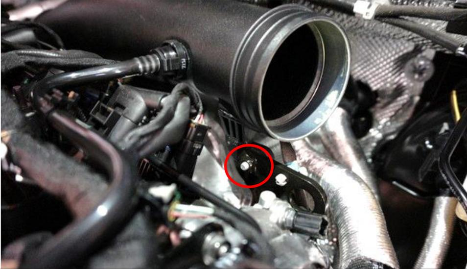
9. Remove the screw securing the Turbo Tube.
