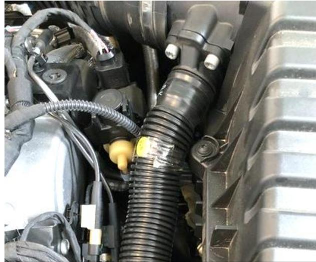
3b. For 2019+ DWNA engines the breather hose is attached onto an adapter with 2 cap head screws. Remove these screws and remove the hose attachment to the airbox.
