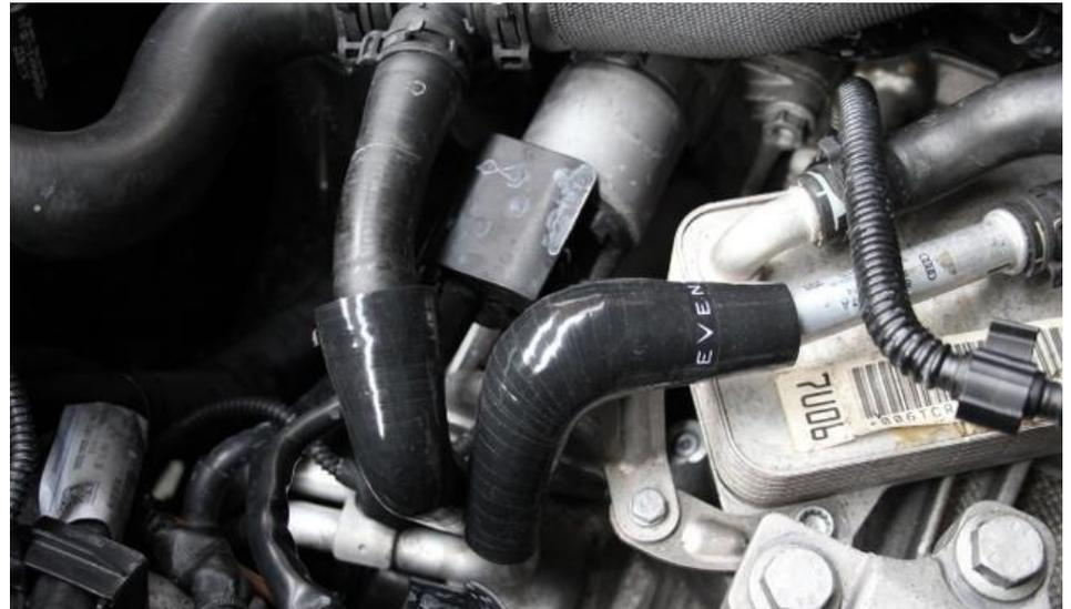
24. The hose will stick up slightly – it is not meant to be completely flush with the metal tube.
