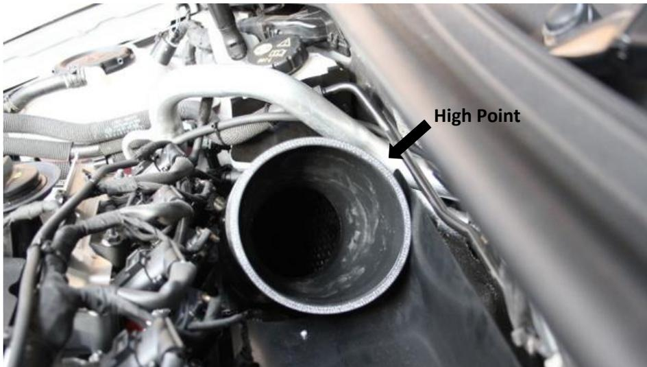
33. Rotate the silicon so that the high point now faces the 2 O'Clock position. Secure it by tightening the hose clamp around the stock inlet.
