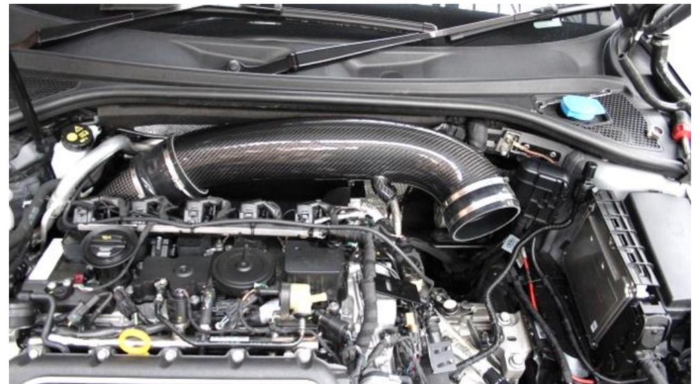
40. Push the carbon tube into the silicon reducer as shown – don't tighten the clamps yet. Optional carbon turbo elbow shown.
