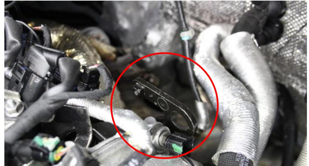
26. The shield and tub bracket are mounted together to the same location at the back of the engine where the OEM tube was fixed (Step 5). If there is a cable attached by a clip to this bracket – remove also.
