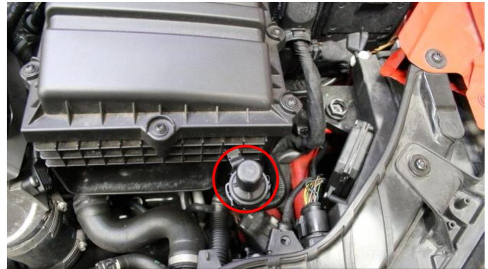
2. Remove the breather pot from the airbox – it is held in place with a panel clip – use a small flat head screwdriver to prise the clip open if required.
