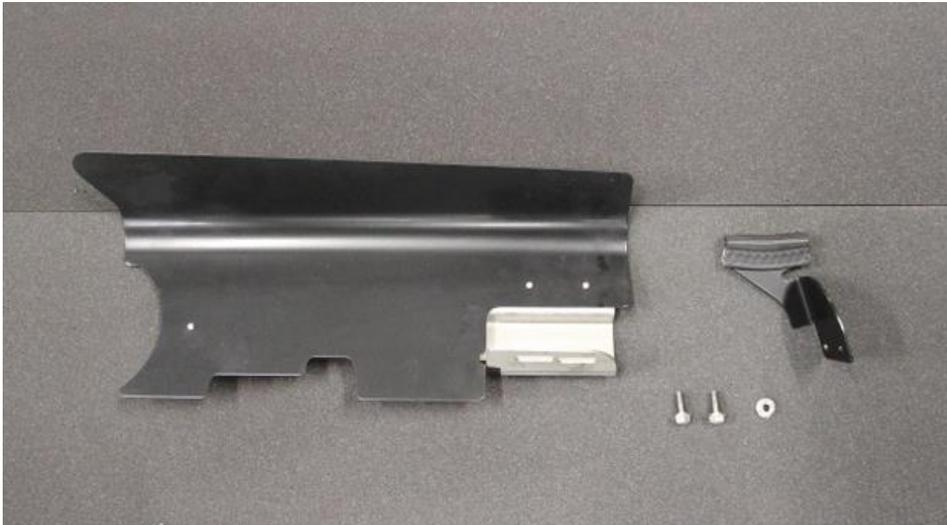
25. Take the heat shield, tube bracket with rubber edge and the 2 supplied M6 Screws with 1 M6 Non Locking Nut.
