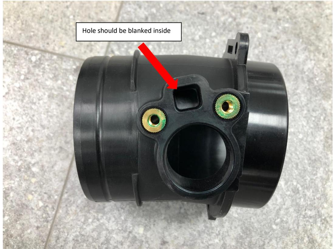
With the breather hose removed you will be able to see this tube connected to the OEM airbox. Please have a look at the square hole as indicated above. This should be blanked off on the inside. So you **SHOULD NOT** be able to see all the way through this square hole. If you can see all the way through this hole and into the tube please **DO NOT** install the intake – contact your Eventuri Dealer.
