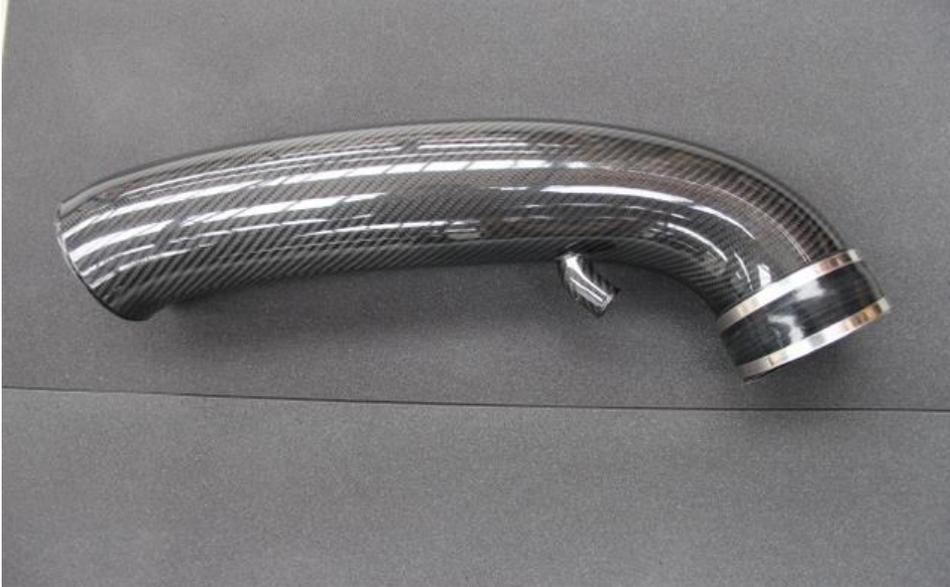
37. Take the carbon tube and place the straight silicon coupler over it with 2 hose clamps.
