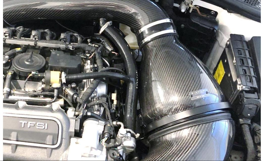
57. Install the breather hose as shown for the 2 variants and secure the hose clamps.
