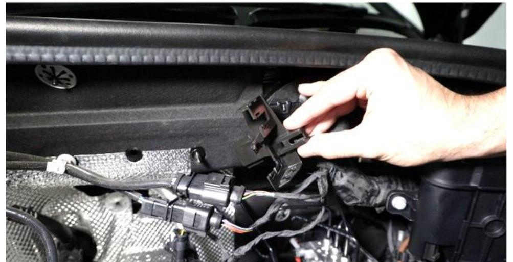
16. Remove the plastic bracket completely.
