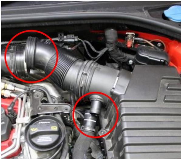
3a. Remove spring clamp from flexi hose at the turbo pipe connection – use an appropriate spring clamp tool. Pull out the flexi hose from the turbo tube. Also remove engine cover and breather hose from the airbox.
