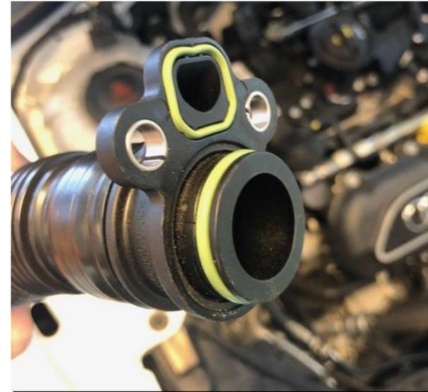
6. Remove the 2 rubber seals from the adapter fitting.
